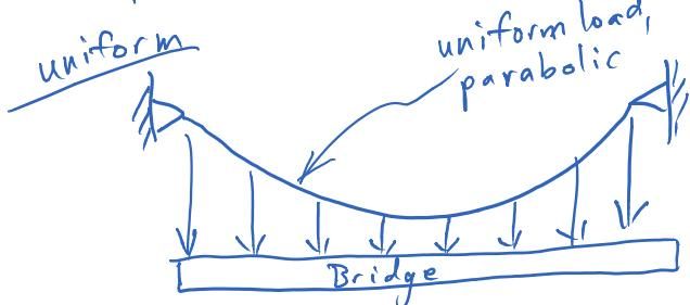
If distributed load is uniform, the cable curve  $y(x)$  will be parabolic
