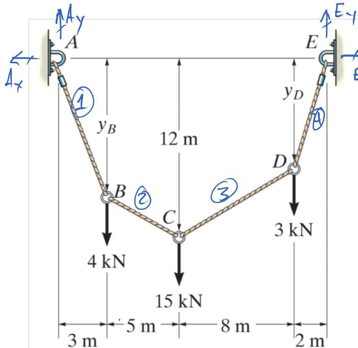
Determine the tension in each segment of the cable shown.
